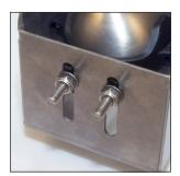
Slotting holes for positioning camera in vertical and horizontal direction.
