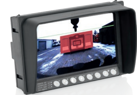
Camera setting: Horizontal line mark. This option shows a reference line on the monitor.
